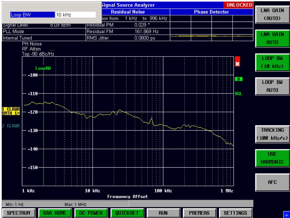
Fig. 5-16 Phase noise measurement result display
